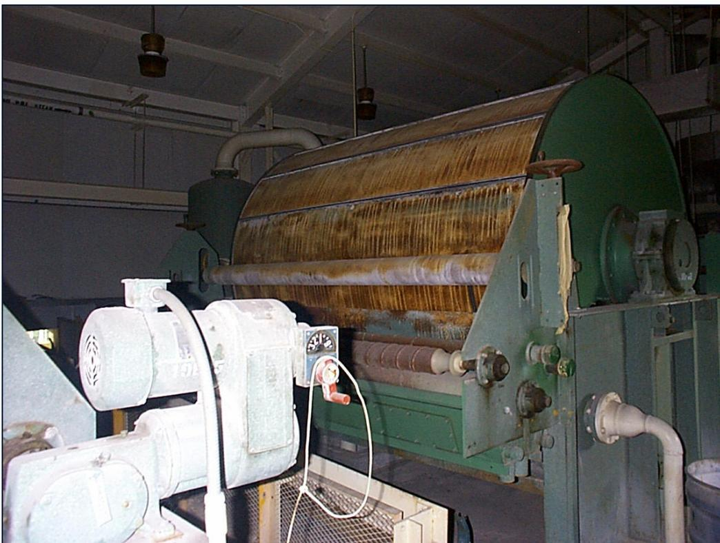
**PHOTO 7: SSA 18 – Unit 18b Vacuum Drum Filter**
